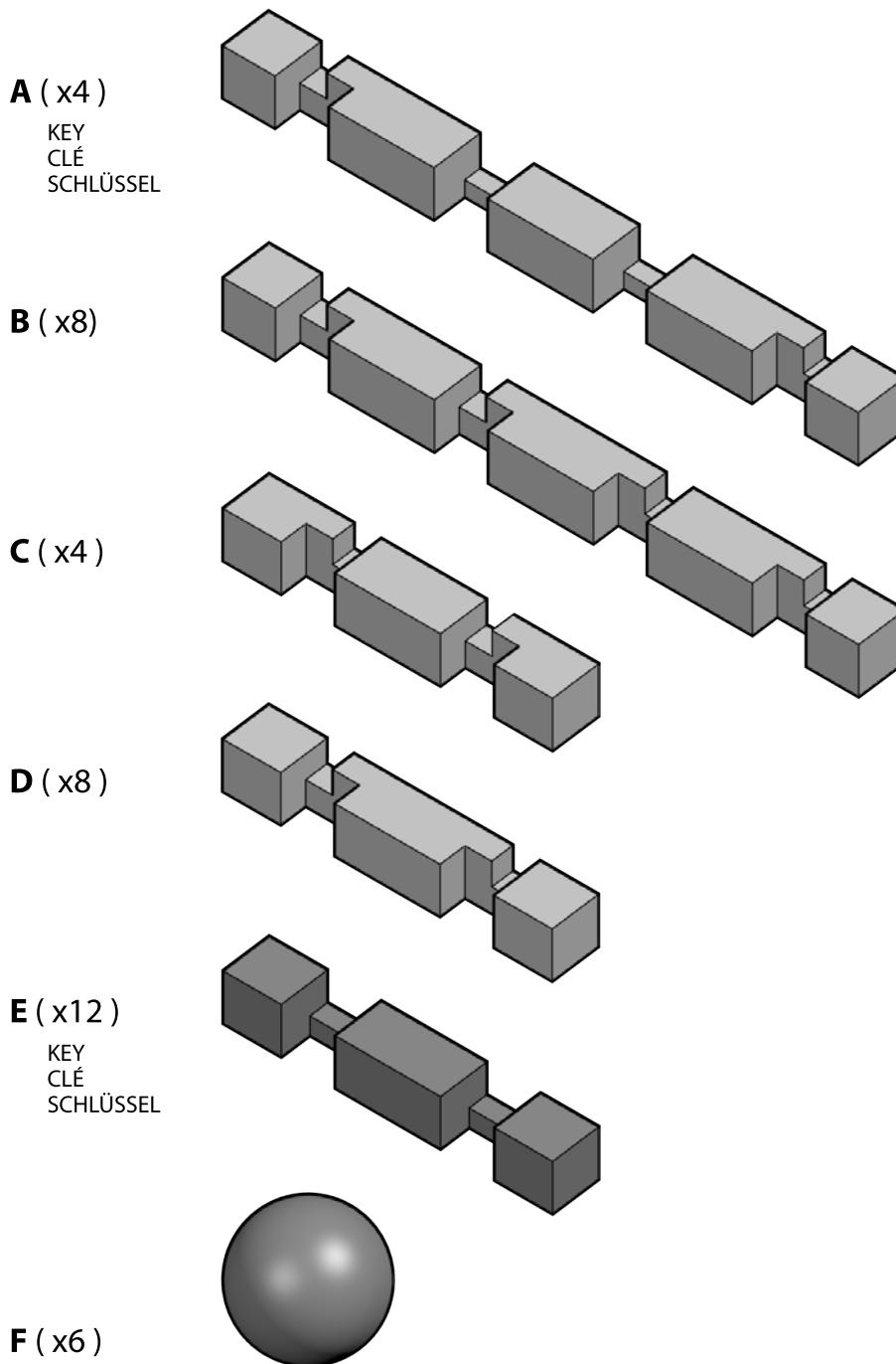
**Attention:** Please note that no force is required to disassemble the Imprisoned Spheres puzzle. Two of the pieces, the so-called "keys" (A, E), can rotate. Knowing this is the trick that allows one to disassemble the Imprisoned Spheres puzzle.
